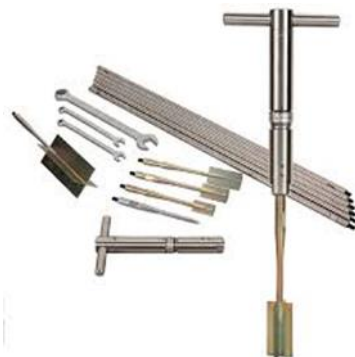
Humboldt Hand Held Vane Shear Test Device
