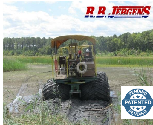
Photo 2: Floating Tire Rig with Full Service, In-situ Geotechnical Testing
